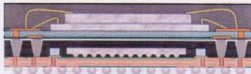
FIGURE 2. Cross-section of joined top and bottom packages, showing through-mold vias as gray columns. Courtesy of Amkor
